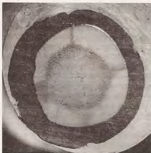
FIG. 5. Cross section of recovered boron nitride core shock processed in PETN at 1.0 g/cm 3 . The dark outer ring is the aluminum tamper, the light inner ring is untransformed boron nitride, and the central gray region is associated with transformed boron nitride.
